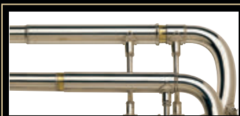
Reversed mouthpipe construction (pictured bottom, standard pictured top) eliminates a step at the main tuning slide and maintains longer taper length, creating a more open feel with less resistance and improved intonation.
